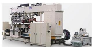
Mash seam welders are used by steel manufacturers for connecting coil in many different processes, including Continuous Galvanizing Lines (CGLs), Annealing & Coating Lines (ACLs), Multi Coating Lines (MCLs), and Continuous Annealing Lines (CALs). 50 to 100 units are typically used in the iron making process. The acid treatment line (CPL) below is a schematic diagram as an example.
