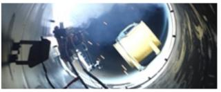
Water pipe welding (carbon steel), automated inner and outer surface welding using touch sensing and arc sensing (all positions) SF-71 1.2mm, CO2 100%(190A ~ 220A/22V ~ 24V)
